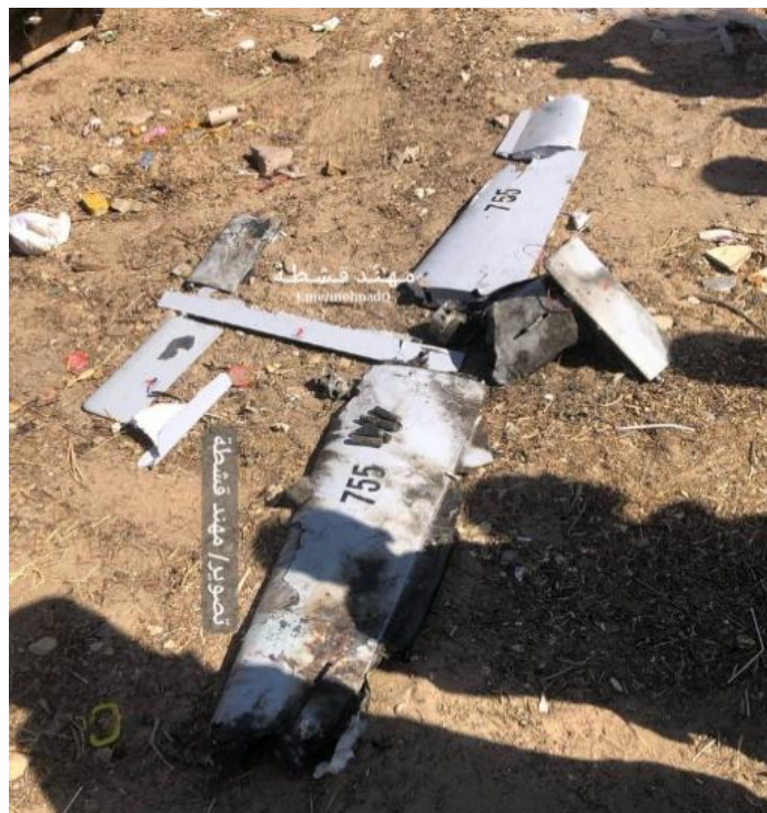
A Skystriker loitering munition identified from debris in Khan Younis, Gaza, 17 April 2025 © Open Source Munition Portal 137
